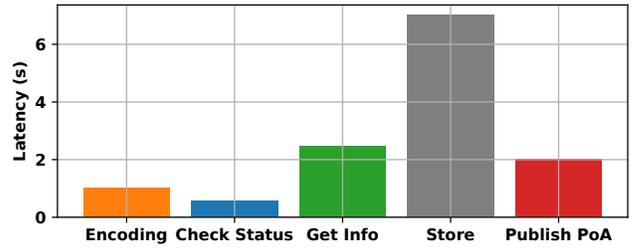
Figure 9: Latency breakdown for small blobs (1KB).
